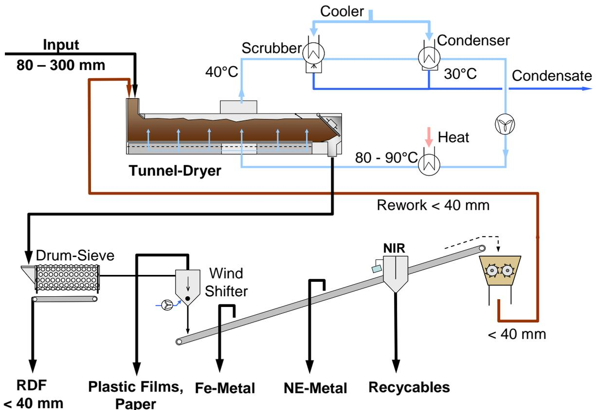
Figure 1: Process flow diagram tunnel dryer with processing
